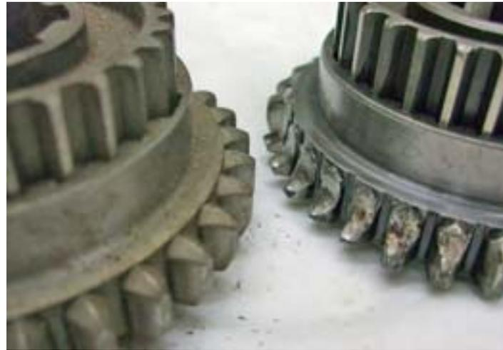
**WARNING!** When handling this gear, be careful not to accidentally push the 1<sup>st</sup> gear ring off the central hub. There are 3 spring-loaded ball bearings ready to launch into outer space if the gear ring is allowed to slide too far. I have been able to re-assemble these using a 'Bisto' jar lid, a jubilee clip and a lot of blue language as well as a large supply of balls and springs!
