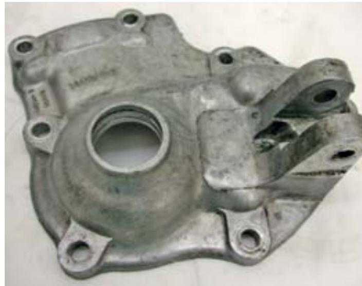
Taking the side cover off the gearbox will expose most of the "innards" for inspection, but be careful not to trap or lose the two plunger springs that will be released. You will be looking for anything obviously awry, broken, chipped or rusty gearwheels. Emulsified (milky) oil indicating moisture or even water, which will have done the bearings and shafts no good at all!
