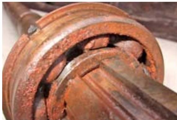
until the resulting bearing play causes premature gear failure
