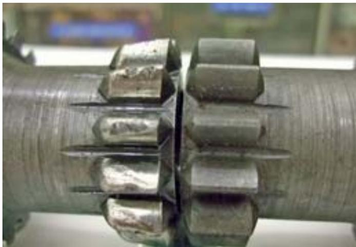
Replacement of the lay gear cluster can present more of a potential noise problem as this affects all of the gears. Incidentally, a noise like an enraged bellowing elephant in 1<sup>st</sup> or reverse gears is normally a sign of wear in the layshaft and bearings.
