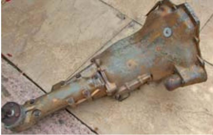
The best bet for buying a second-hand gearbox to fit "as is" is to obtain one from a recently scrapped car where it has lain in the frame horizontally full of oil.
